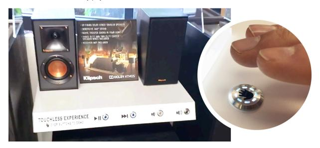
New Klipsch Audio displays use AirSelect touchless sensors by Ascentic Retail Engineering to protect consumers from the spread of pathogens. The hand symbol invites users to interact without touching, and response lights confirm the user's actions.
